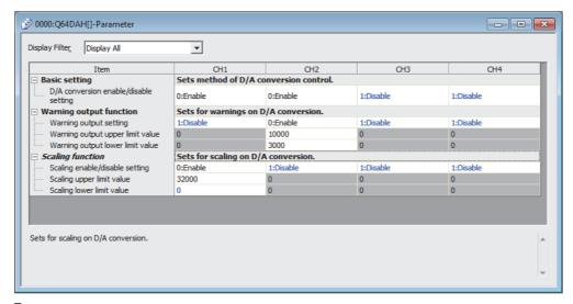
**5.** Display the auto refresh setting window for the Q64DAH and configure the setting as follows. When creating a program without using parameters of an intelligent function module, skip this procedure.
