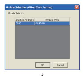
1. Select the module to configure the offset/gain setting, and click the button.
