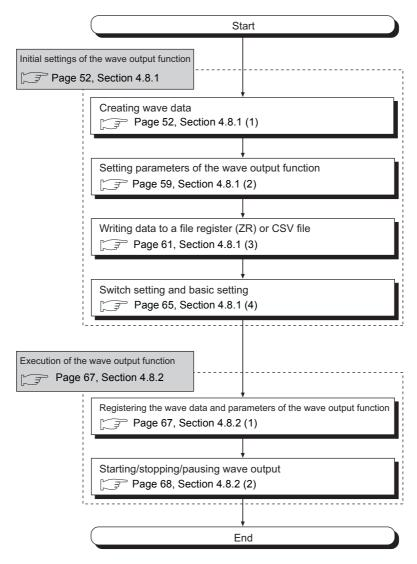
The wave data creation and parameter setting of the wave output function can be executed easily with "Create Wave Output Data" of GX Works2. These setting contents are saved in the file register (ZR) of the CPU module or in a CSV file and registered to the buffer memory of the D/A converter module with the function block (FB) for the wave data registration.
