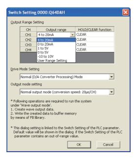
3. Set "Output mode setting" to "Wave output mode (conversion speed: 50µs/CH)" or "Wave output mode (conversion speed: 80µs/CH)".
