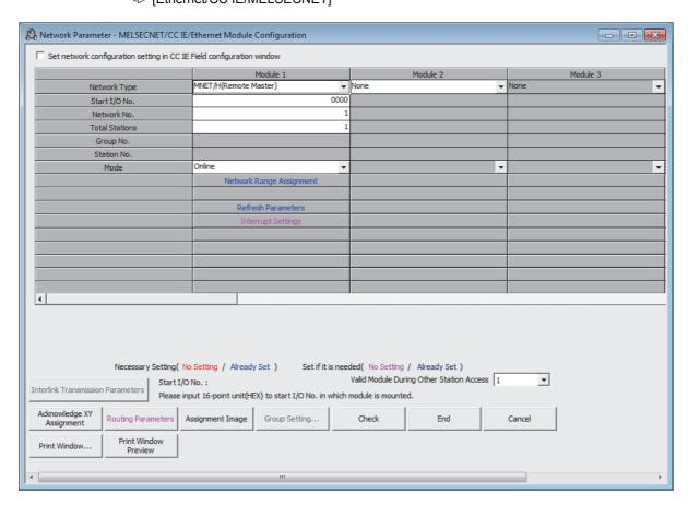
3. Display the network range assignment setting window and configure the setting as follows.
