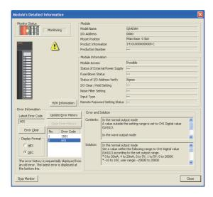
"Module's Detailed Information" of the D/A converter module is displayed.
