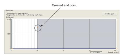
To delete the end point, move the mouse pointer to the point. Then select "Delete end point" from the right-click menu. When the mouse pointer is on the end point, the display of the mouse pointer is changed to +.
