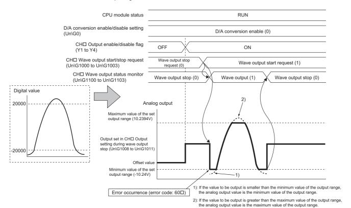
In addition, when the digital value out of the range is set and the error (error code: 60 ) has occurred, correct the value to the one within the range and turn on and off Error clear request (YF).
