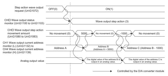
Set Step action wave output request (Un\G1072) to ON (1) to set the wave output status to the wave output step action.
