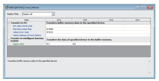
6. Write the set parameters to the remote I/O module and reset the remote I/O module.
