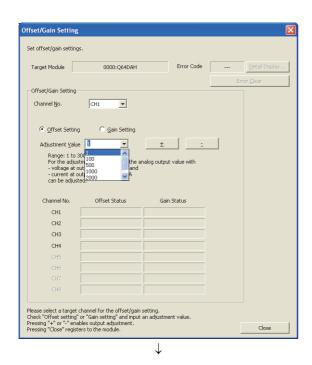
The adjustment amount of the offset value or gain value can be selected from "1", "100", "500", "1000", "2000", and "3000" or it can be set by inputting any value (1 to 3000).
