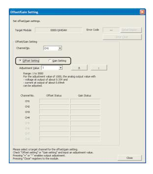
**4.** Use the radio button to specify whether the offset setting or gain setting.
