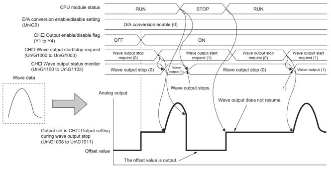
Wave output starts when the value set in CH□ Wave output start/stop request (Un\G1000 to Un\G1003) is changed from Wave output stop request (0) to Wave output start request (1).
