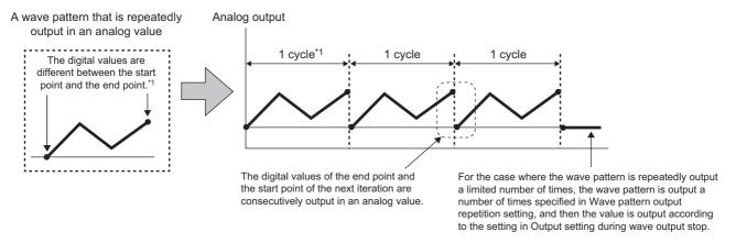
\*1 The output cycle of a wave pattern is calculated by the following formula.
